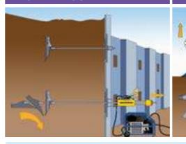
A tensile load is applied to the attached tie bar or tendon. This rotates the anchor into the locked position for maximum load holding capacity. The anchor is then proof tested to the designed loading requirements before the top termination is fitted, as specified by the civil or structural engineer.
